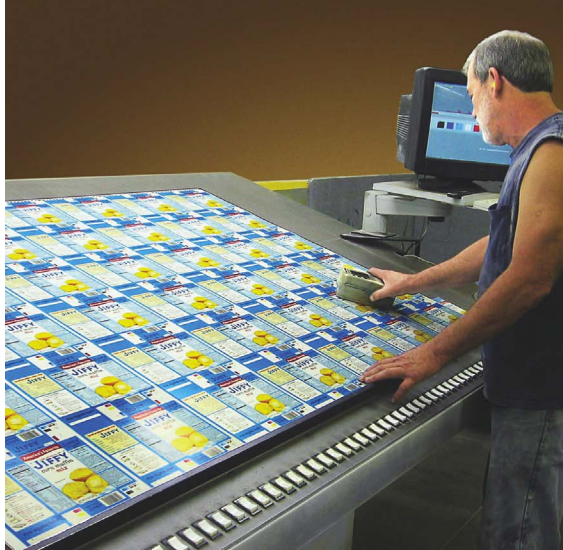
Don Whitney, a pressman at C&S Carton, examines Jiffy carton ink-color densities produced by the new control.
