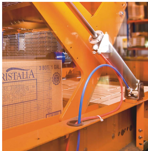
Case stops in the palletizer's row-forming area space the cases properly while a pusher bar transfers them one row at a time to a layering apron.
