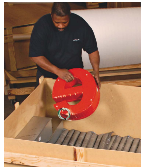
Continuous foam tubing pads large sign letters packed in wooden crates. The Insight foam system allows operators to pack more of the crates in less time.
