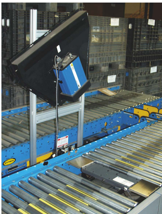
RFID stations with a control console and scanner, above, are in place in the 'induction areas' at the end of each packaging line at Knoll Mfg.'s production facility.
