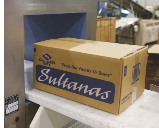
One of the new metal detectors in action, inspects cases of Golden Boy's Sultan's raisins. The system tracks the tiniest of metal contaminants.
